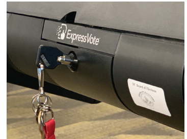
Barrel Key unlocks the front panel
